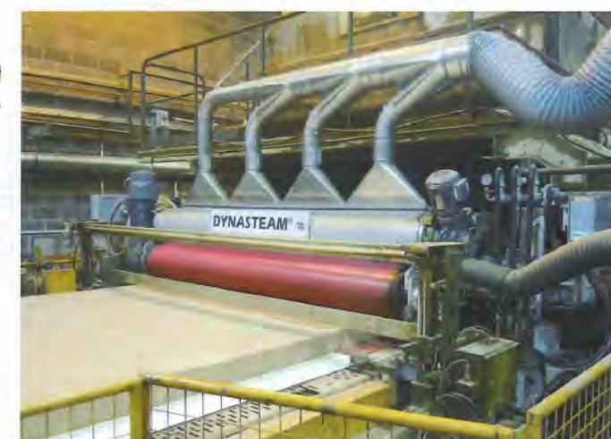
Above left: The woodchip pressed pallet business is going well Above right: The DynaSteam mat pre-heating system
