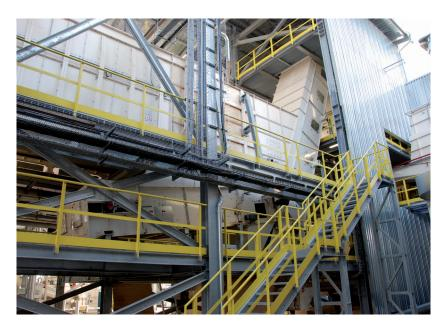
The picker rolls located at the front of the strand bin ruin and break the strands leading to consequent issues with OSB panel quality and excessive resin consumption. IMAL has designed a solution which resolves this problem by eliminating the picker rolls from the bin. The strands are continually metered to the continuous scale and blender by a system of inclined belt conveyors, and controls and levels mounted on the bin.
