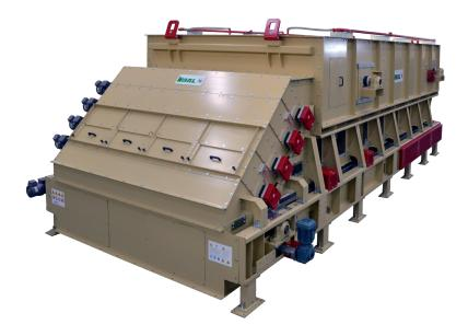
The BCD.OSB have been specifically designed to meter flow of strands. It consists of a belt with a storage/levelling area located at the top of the machine and a weighing area at the front end. Another important function of this scale is to create a mat of strands with a controlled konstant height at discharge.
