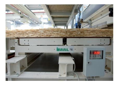
The system assesses mat weight at forming line outlet, so that the forming machines or the levelling scalper can be adjusted in order to obtain a constant weight per square meter value to coincide with that previously set.
