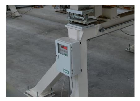
This weighing system is composed of load cells, of a suitable load, to support the conveyor unit. An IMAL electronic digital amplifier supplies the voltage, appropriately filtered and adjusted, to the cells, and amplifies the proportional weight signal. This value can then be transmitted to other quality control systems, like the thickness gauge, so that density may be calculated.
