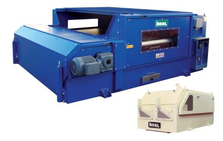
• The small size of the BT or BN model means that they can be installed in any plant • BT or BN model are particularly suitable for all plants where continuous material weighing is required to assist in on going adjustments and controls. The material is conveyed on a belt connected to an electronic weight transducer. The signal is converted by an electronic amplifier that instantly displays the weight in Kg/min or lb/min.
