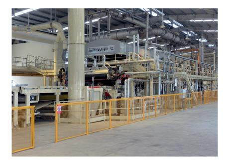
Continuous press provided with integrated steam injection unit (Imal Dynasteam). The mat enters the continuous hydraulic hot press (DynaSteamPress) where it is pressed between two rotating steel belts which transfer pressure and heat to the mat.
