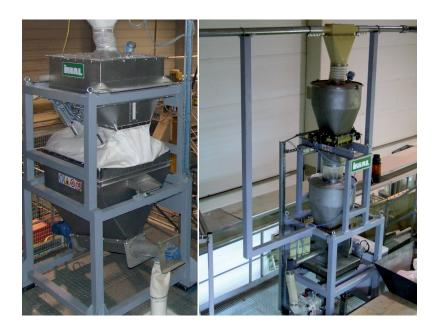
Fire retardant boards are produced with the addition of powder additives. Furthermore, boards with low formaldehyde emission are also produced using pearl urea which is dosed and pulverized before it is added to the work process. IMAL has designed powder conveying and dosing systems for these applications which are easily suited to all kinds of plants.
