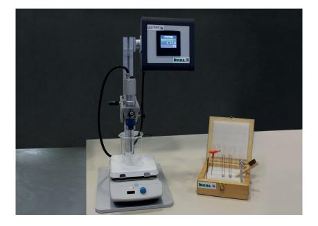
The Geltimer has been designed to measure the gel time of the resin delivered by the supplier and the gel time of the glue mix applied in the blender and the blow line.
