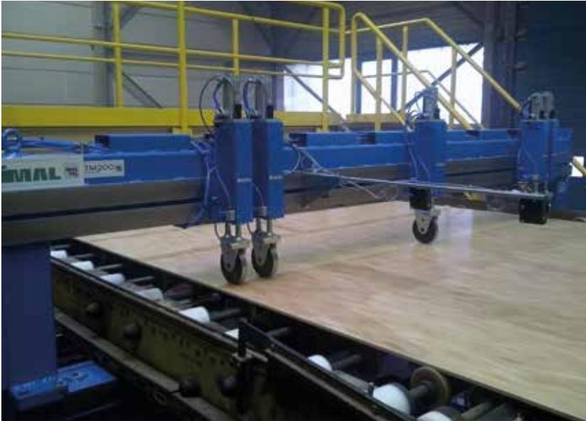
The TM200 system has been designed for the on-line measurement of thickness, weight and density (when used in conjunction with the weighing scale).
