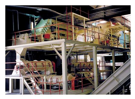
Extended mixing time and the double blending of particles and glue have provided good results in many particleboard plants. Improved board properties, greater consistency and considerable reduction in glue consumption are just a few examples of the benefits had with this method.
