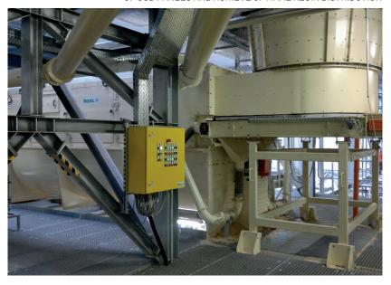
IMAL has designed a solution where acceleration rolls, installed at the outfeed to the scale and prior to the blender, create a very fine curtain of strands and the resin (ie. MDI, MUF, PF or MUPF) is then "painted" at high pressure over the strands as they fall inside the chute. During the next phase the strands are mixed and blended by a special mixer with a shaft that rotates at low speed, specially designed to achieve a perfect blend.
