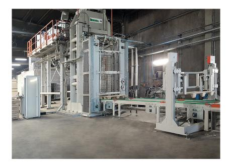
The single-opening press for pallet production is able to produce all kinds of pallet from all varieties of wood-based raw materials.
