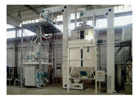
Our Cooler refresh the Pellets by using a forced air counter flow. Pellet will be dosed inside the machine by a R-Valve who ensure the no dust propagation in the rounding area.
