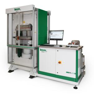
The laboratory press is able to produce sample boards for testing purposes, with adjustable specific pressure and adjustable temperature for binder curing. The PL100 Laboratory Press is produced in a standard 600 x 600 mm version but other sizes may be evaluated upon request.
