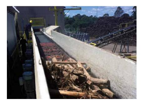
Together with a Debarking System or alone embedded in Logs feeding line, the Roller Discharge give you the highest capacity of bark and residues evacuation out of the process line. With different designs and several association of extremely heavy duty rollers, the Roller Discharge supply high capacity and performance in cleaning. The advance design of the mechanical elements, allow an easy maintenance procedure and low energy demand ratio.
