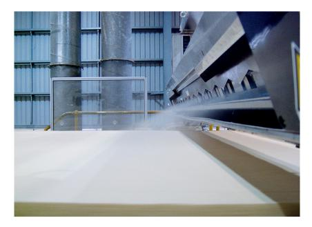
The TS100 system has been designed for damping the top and bottom surfaces of the mat as it travels along the forming line.
