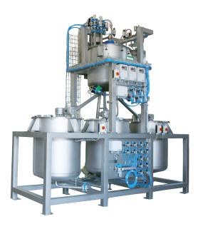
The WINGRAV9 gravimetric system designed for the preparation of resin mixtures for impregnation lines may be configured to suit a wide range of applications and requirements. The pre-programmed software may in fact be adapted to accommodate a large number of components, additives and utilities.
