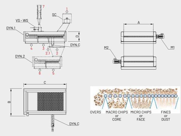
SC = DOSING SCREW CONVEYOR DYB.1 = 1-DECK DYNASCREEN DY.2 = 2-DECKS DYNASCREEN
