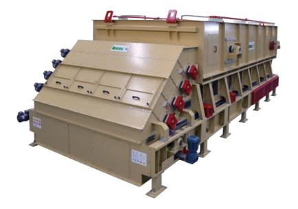
The BCD.OSB has been specifically designed to meter flow of strands. It consists of a belt with a storage/levelling area located at the top of the machine and a weighing area at the front end. Another important function of this scale is to create a mat of strands with a controlled constant height at discharge.
