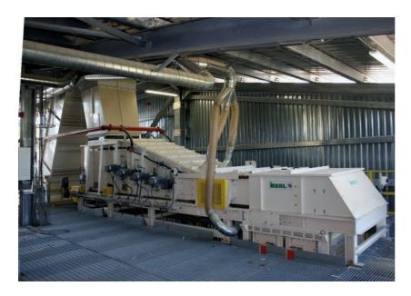
The BCDS metering bins have been specifically designed to meter low to medium flows of light and dusty material, enabling a perfect flow adjustment even in cases of irregular material feed.
