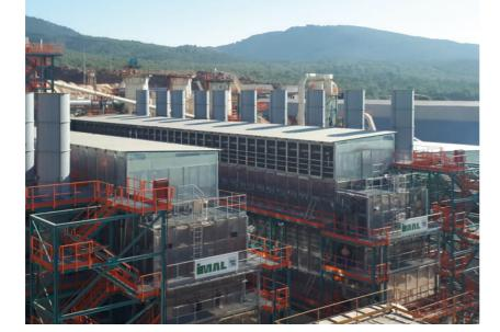
Belt dryers are able to dry particles up to a moisture content of less than 1%. They may be used in PB and OSB panel production, PELLET production, PAL-LET BLOCK production.
