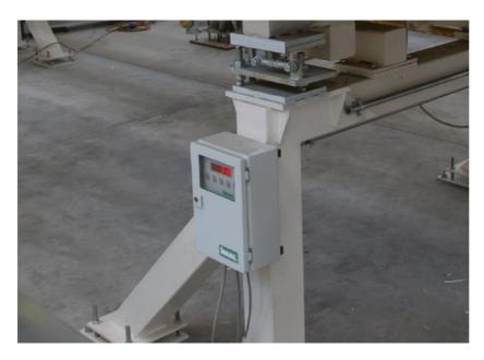
The BPP is a scale that has been designed for the continuous weighing of raw boards.
