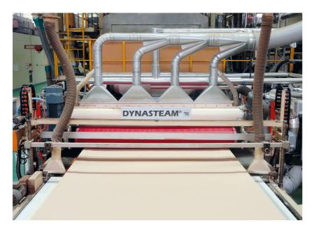
The DYNASTEAM® system has been designed to inject a continuous pre-set quantity of steam onto the top and bottom surface of the mat, or bottom surface only, depending on the application, as it is fed into the press.
