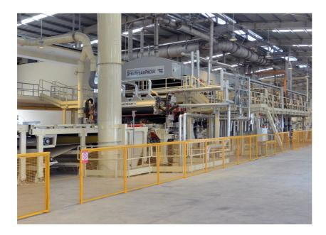
DYNASTEAMPRESS is a continuous press provided with integrated steam injection unit (Imal Dynasteam). The mat enters the continuous hydraulic hot press (DynaSteamPress) where it is pressed between two rotating steel belts which transfer pressure and heat to the mat. The hydraulic units control and adjust the pressure in the various areas of
