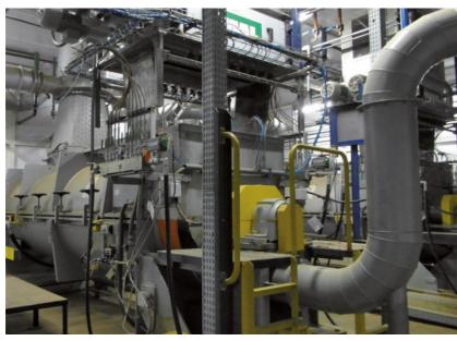
FB is a high-pressure fibre resination technology designed to significantly reduce resin consumption in the manufacture of MDF panels.
