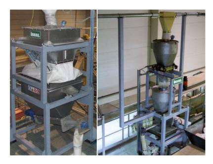
Fire Retardant / Powder Urea Dosing System is a pre-assembled unit designed for dosing powder products.
