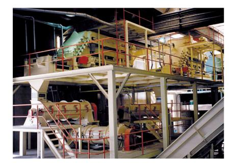
IPL9000 are dual glue blenders designed to be installed in an L-shape configuration. Extended mixing time and the double blending of particles and glue have provided good results in many particleboard plants. Improved board properties, greater consistency and considerable reduction in glue consumption are just a few examples of the benefits had with this method.
