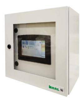
MULTICOMP BCD is an amplifier unit that has been designed to amplify the load cell signal and calculate the flow rate of the BCD scale, making this data available on the display and via a 4-20mA analogue signal.
