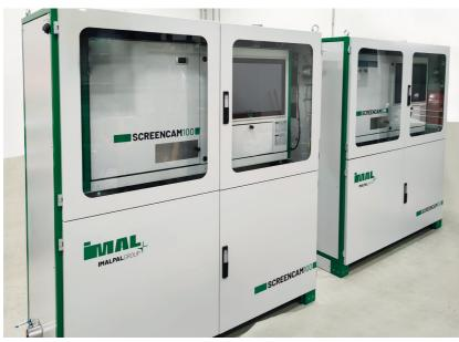
The application of optical technology in the ON LINE SCREENCAM 100 permits an accurate measurement of the dimensions of the particles directly online in a completely automatic way, with elevated repeatability and rapid response times, new results are obtained every couple of minutes.
