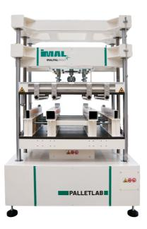
PALLETLAB is a machine for testing the quality and mechanical characteristics of wooden pallets in various conditions and then processes the results obtained.
