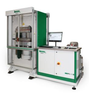
The laboratory press is able to produce sample boards for testing purposes, with adjustable specific pressure and adjustable temperature for binder curing. The PL100 Laboratory Press is produced in a standard  $600 \times 600$  mm version but other sizes may be evaluated upon request.
