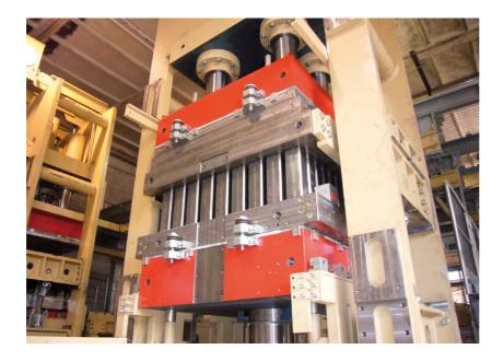
The single-opening press for pallet blocks production is able to produce all kinds of pallet blocks from all varieties of wood-based raw materials.
