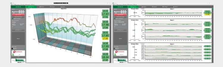
The TM200 – LEV version is also available for installation on the sanding line. This version differs from the standard version in that the system is able to control measuring points distributed over several beams (up to 4 beams for a total of 48 measuring points), with the measurements conveniently displayed on the same monitor.
