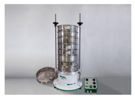
VM100 is an electro-magnetic impulse operated Sifter, controlled by a separate micro-processor with the following functions:
