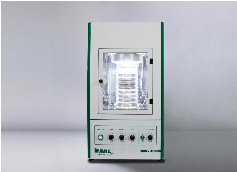
The VU200 has been designed to screen out products like sawdust, chips, and wood fibre, in relation to particle size. By applying an acoustic pressure of adjustable frequency and intensity, the material is dry-sieved and collected in calibrated screens which are positioned in decreasing order. By weighing each sieve, the operator may calculate the percentage of the single granulometries, and obtain numerical information on the composition of the material used.
